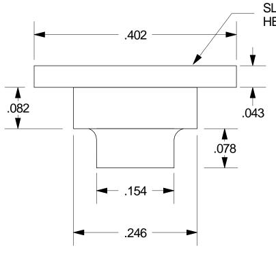
SLIGHT RINGS ON HEAD / UNDER HEAD TO CONTROL METAL FLOW
